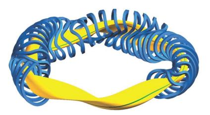
In stellarators, shaping of the magnetic coils to confine the plasmas
