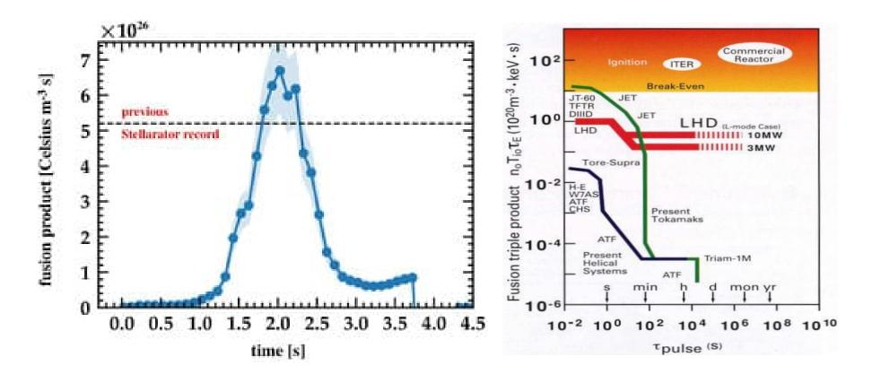
• Fusion product  $6x10^{26}$  Celsius m<sup>-3</sup> s  $\approx 0.5x10^{20}$  keV m<sup>-3</sup> s was obtained with T<sub>i</sub> > 3 keV and n<sub>i</sub> =  $0.8x10^{20}$  m<sup>-3</sup>
