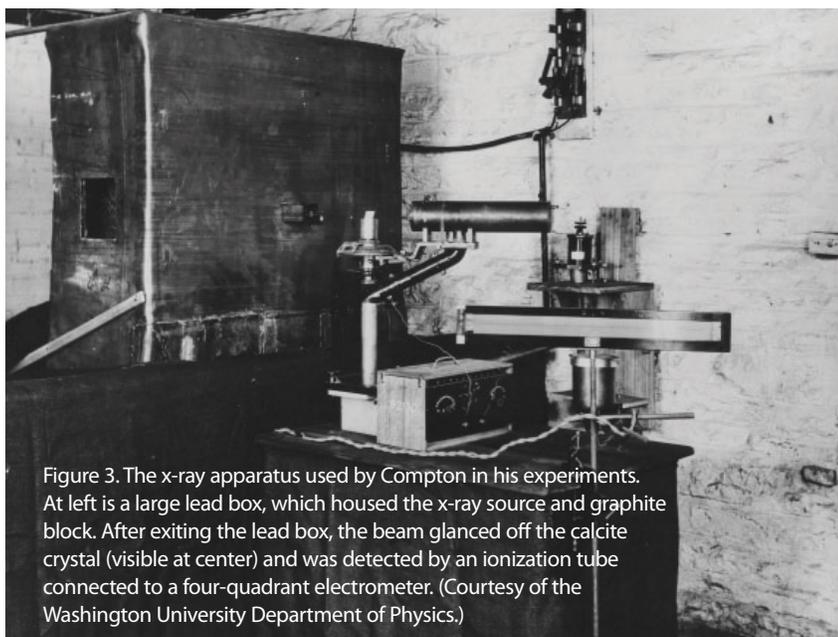
Figure 3. The x-ray apparatus used by Compton in his experiments. At left is a large lead box, which housed the x-ray source and graphite block. After exiting the lead box, the beam glanced off the calcite crystal (visible at center) and was detected by an ionization tube connected to a four-quadrant electrometer. (Courtesy of the Washington University Department of Physics.)
