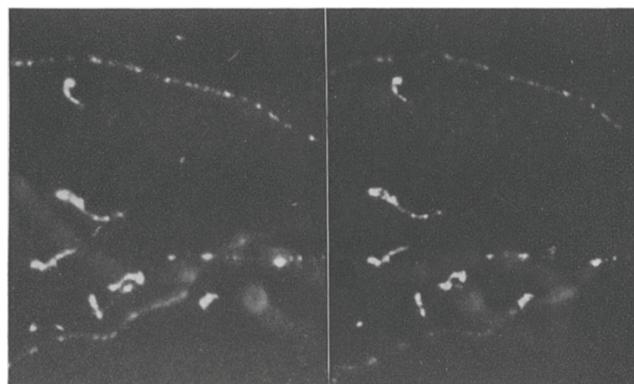
**FIGURE 5. SO-CALLED FISH TRACKS**, or spherical clouds with small tails, photographed by Charles Wilson in his cloud chamber and published in his 1923 paper. Wilson suggested in that article that the tracks were left by recoiling electrons from Compton scattering. (Reproduced from ref. 15.)
