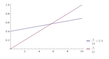
Figure 1: Fuel cell and battery system operating time dependency on system size (y axis system size (litres), x-axis system lifetime (hours)). Blue line is the fuel cell system and red line the battery system.
