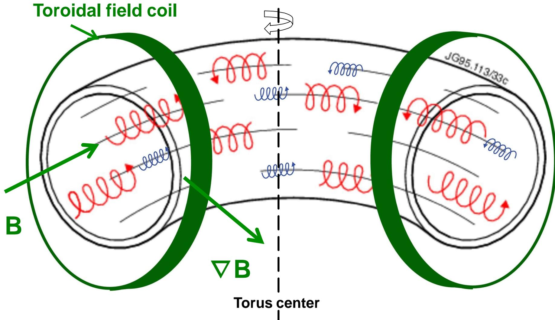
A purely toroidal system will lead to (up-down) charge separation and  $\nabla B$  radial outward drifts
