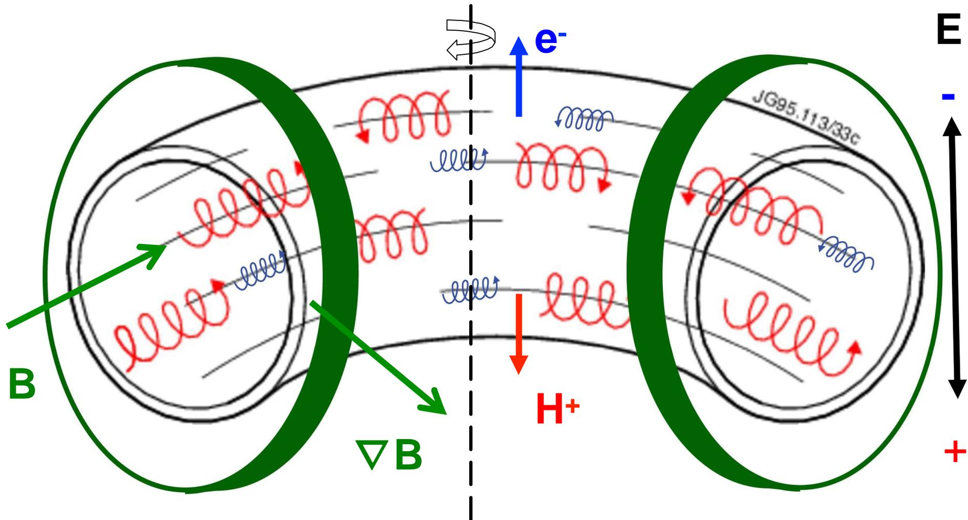
⇒ Short-circuit of up-down charge separation is required
