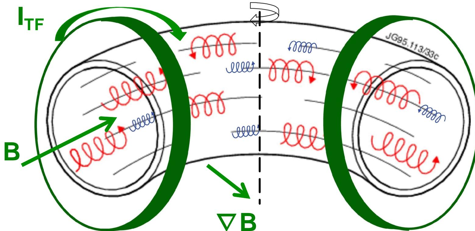
Toroidal magnetic field strength by Ampere's law:
