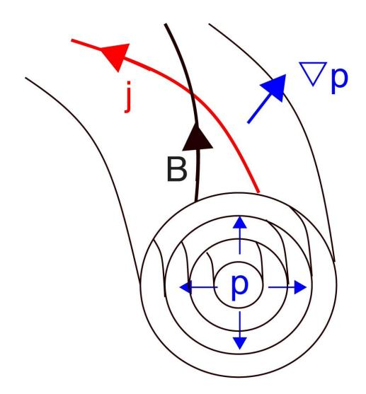
Stationary equilibrium determined by balance between plasma pressure and magnetic force (Grad- Shafranov equation):
