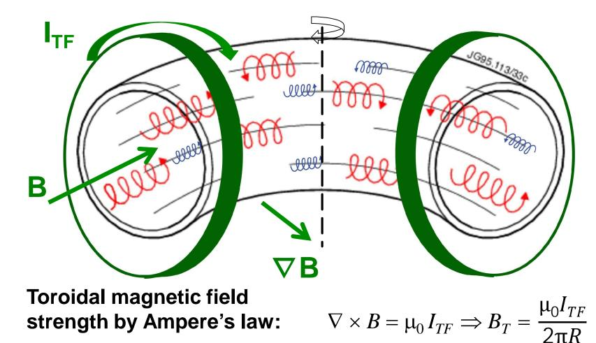
$$\frac{\Delta B_T}{B_{T0}} = \frac{2R_{minor}}{R_0} \approx \frac{3}{4}$$
