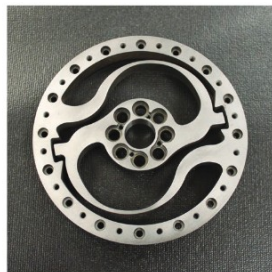
Torsional spring of series elastic actuator
