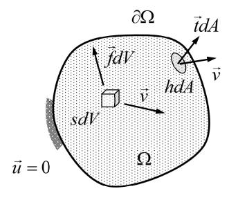
Constitutive equations of the form  $\vec{q}(\theta)$  (heat flux) and  $\vec{\sigma}(\vec{u},\theta)$  (stress) are needed for a closed equation system in terms of displacement and temperature.
