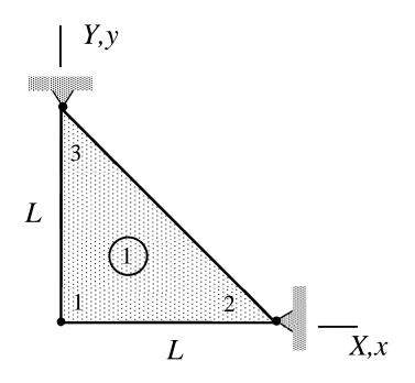
• The non-zero displacement components are  $u_{x1} = u_{X1}$  and  $u_{y1} = u_{Y1}$ . The linear shape functions  $N_1 = (L - x - y)/L$ ,  $N_2 = x/L$  and  $N_3 = y/L$  can be deduced from the figure. Therefore, approximations are
