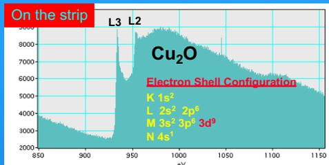
Note: Electron energy loss spectrum (EELS) from the fresh Cu foil.
