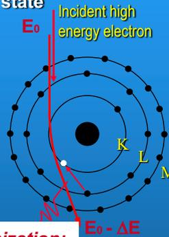
*The energy loss in incident electrons give rise to ionization;
