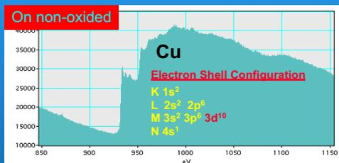
Upon oxidation, some 3d electrons in Cu are transferred to the oxygen, leaving unfilled states, and the white line appears in the oxide spectrum.
