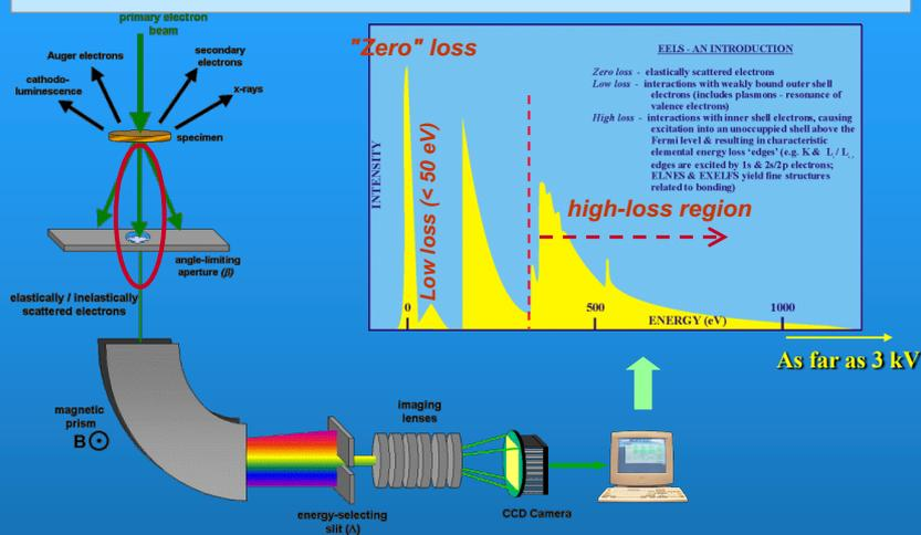
EELS collects electrons that experience energy losses after "inelastic" interaction with the specimen, then display their energy distribution.
