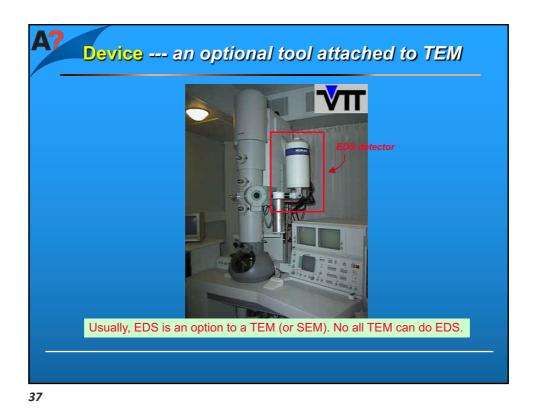
Device --- an optional tool attached to TEM Detector: generates a • charge pulse Computer proportional to X-ray energy, and then converted to a voltage. Electronic device: amplifying and processing weak signal Charge Energy X-ray pulse **Pulse** Detector processor data analysis and display 38
