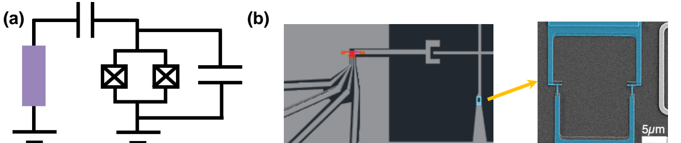
FIG. 1. Exemplary quantum circuit for analysis. (a) Circuit diagram. On the right side a SQUID (superconducting quantum interference device) composed of two Josephson junctions. This element is capacitively coupled to a resistive element on the left. (b) The actual on-chip circuit. The coupling capacitor is the fork-like structure in the middle, and the SQUID is zoomed out in blue on the right. The resistive element is contacted by four NIS tunnel junctions to control and measure temperature, on the left.
