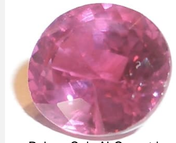
Ruby – Cr in \text{Al}_2\text{O}_3 matrix
