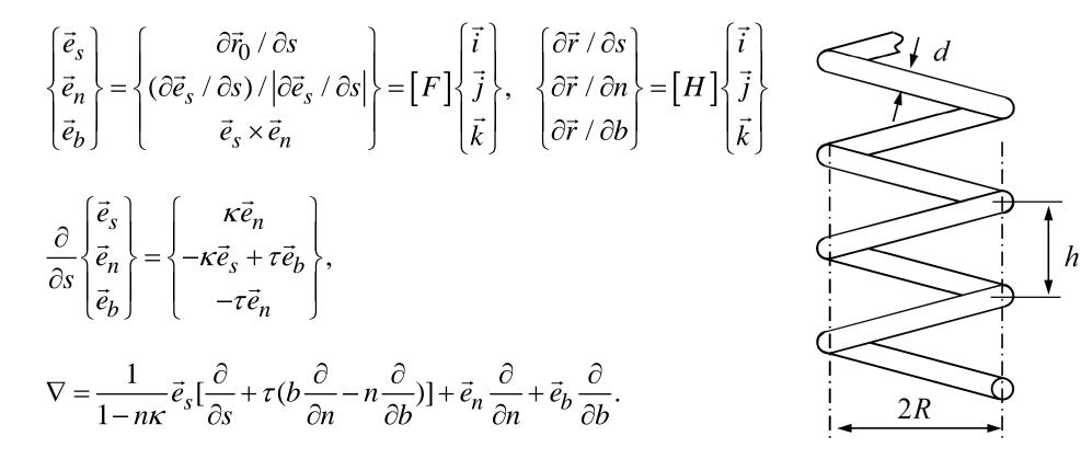
Beam (s,n,b) coordinate system is curvilinear and orthonormal. Therefore the matrix of the basis vector derivatives is anti-symmetric (why?) and expressible in form (Serret-Frenet formulas in literature)
