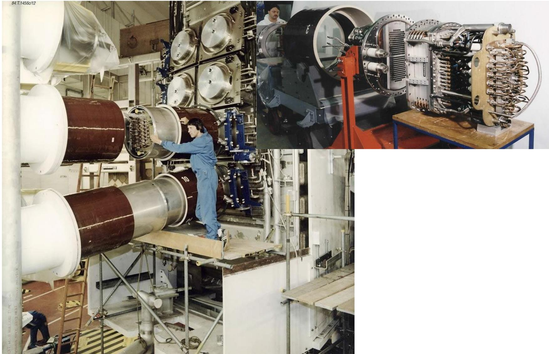
The JET neutral beam (drift) ducts have a height and width of about 0.8 m x 0.2 m
