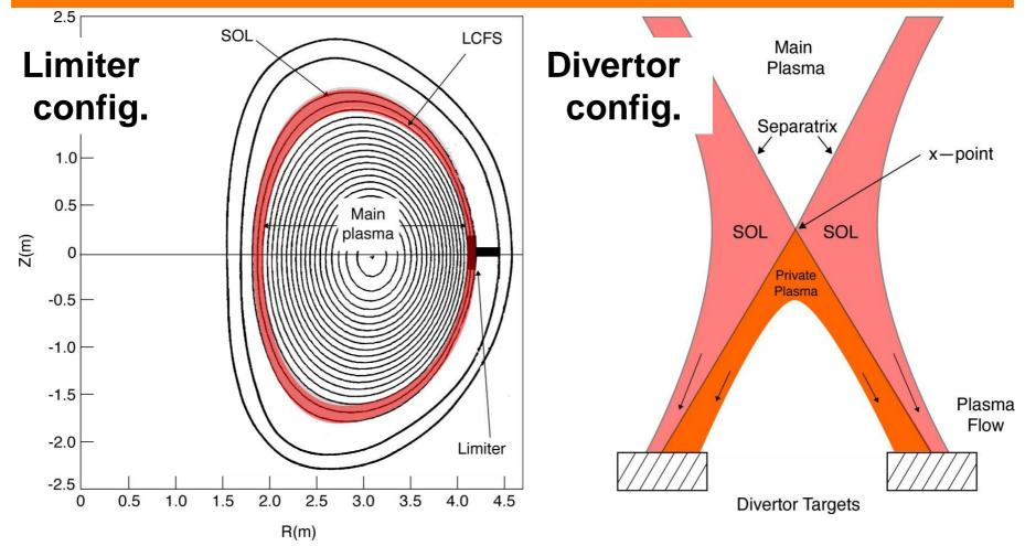
Isolation of divertor from main chamber by adding coils at the bottom of device to produce magnetic null
