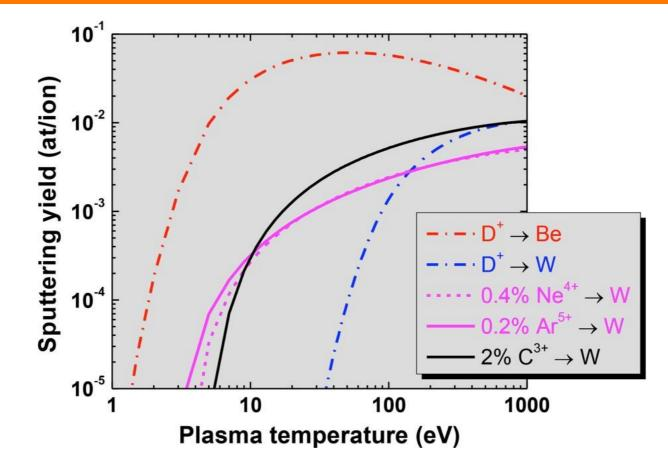
For neon and argon impinging on tungsten, already less than 0.5% is sufficient to drop E<sub>thresh</sub> from 35 eV to 5 eV
