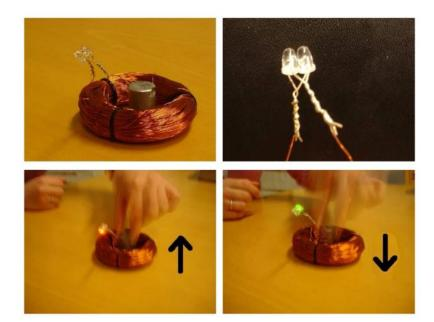
Moving circuit in static magnetic field
