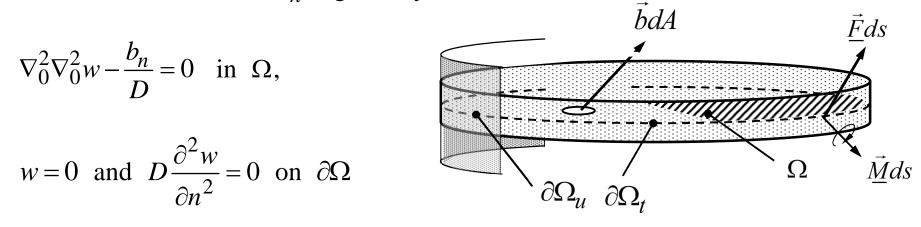
in which  $D = \frac{Et^3}{12(1-v^2)}$  is the bending stiffness of the plate and  $\nabla = \nabla_0 + \vec{e}_n \frac{\partial}{\partial n}$ .
