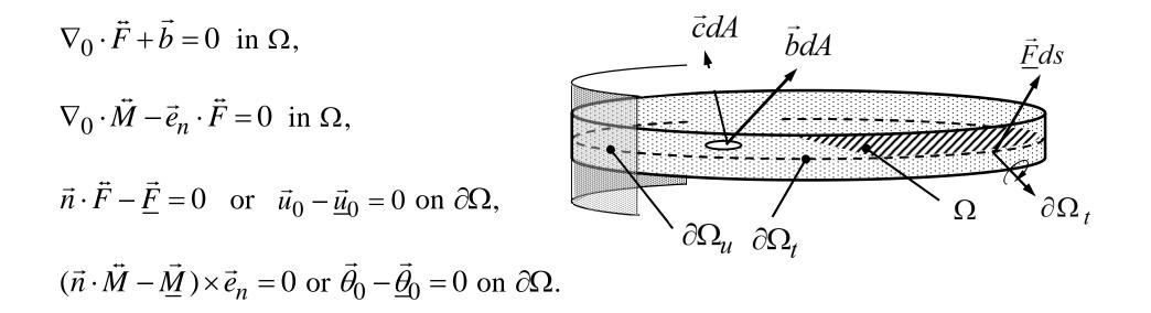
Stress resultants are symmetric so that  $\vec{F} = \vec{F}_c$  and  $\vec{M} = \vec{M}_c$ . Constitutive equations  $\vec{M} = \vec{M}(\vec{u}_0, \vec{\theta}_0), \ \vec{F} = \vec{F}(\vec{u}_0, \vec{\theta}_0)$  are needed for a closed equation system!
