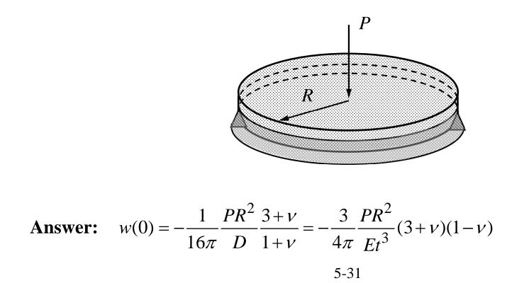
Let us consider first solution on an annular domain of outer radius *R* which is simple supported on the outer boundary and loaded by constant distributed force  $Q = -P/(2\pi\epsilon)$  on the inner boundary  $r = \epsilon$ . Assuming rotation symmetry, the bending mode equilibrium equation and the boundary conditions simplify to
