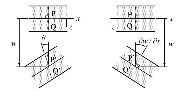
**Kinematic assumption:** Line segments perpendicular to the mid/reference-plane remain straight in deformation (Reissner-Mindlin) and perpendicular to the mid-plane (Kirchhoff). Then, line segments move as rigid bodies according to  $\vec{u} = \vec{u}_0 + \vec{\theta}_0 \times \vec{\rho}$ .
