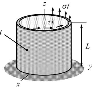
**Answer:**  $N_{zz} = \sigma t + b_z(L-z)$ ,  $N_{z\phi} = \tau t + b_\phi(L-z)$ , and  $N_{\phi\phi} = -b_n R$
