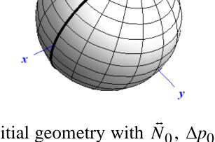
**NOTICE**. Linear elasticity theory assumes an equilibrium initial geometry with  $N_0$ ,  $\Delta p_0$ , and  $R_0$ . The aim is to find the new equilibrium  $\vec{N}$ ,  $\Delta p$ , and R due to the change in pressure. Here, displacement gives the change in radius due to the increase in the pressure difference.
