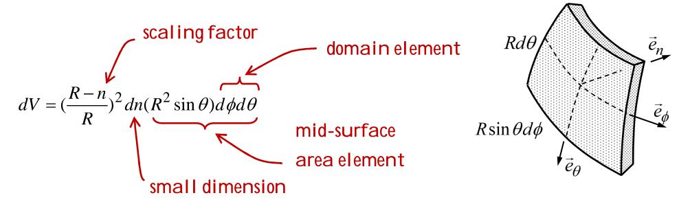
The scaling factors for the area elements depend on the direction of the boundary  $\vec{n}$  (the unit outward normal vector), curvature of the mid-surface  $\vec{\kappa}$ , and normal coordinate n.
