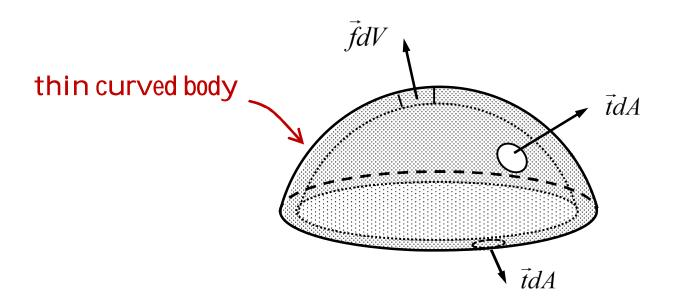
**Kinematic assumption:** Straight line segments perpendicular to the mid-surface remain straight in deformation (Reissner-Mindlin) or straight and perpendicular to the mid-surface (Kirchhoff) in deformation, so  $\vec{u} = \vec{u}_0 + \vec{\theta}_0 \times n\vec{e}_n = \vec{u}_0 + n\vec{\omega}_0$ .
