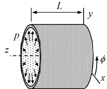
7. Consider a simply supported (long) circular cylindrical shell of radius  $R$ , thickness  $t$ , and filled with liquid of density  $\rho$  in cylindrical  $(z, \phi, n)$  coordinates. Determine the mid-surface stress resultants  $N_{\phi\phi}$ ,  $N_{z\phi}$  and  $N_{zz}$  by assuming that there are no axial forces at the ends of the shell and bending deformation is negligible. (J.N.Reddy: Example 11.3.1)
