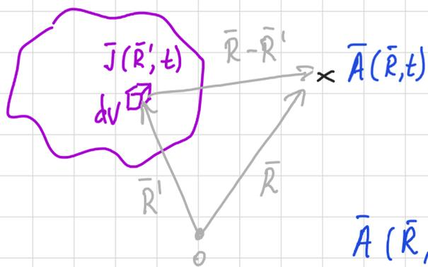
$$\bar{A}(\bar{R}, t) = \int_V \frac{\mu_0 \bar{J} \left[ \bar{R}', t - \frac{|\bar{R} - \bar{R}'|}{v} \right]}{4\pi |\bar{R} - \bar{R}'|} dV'$$
