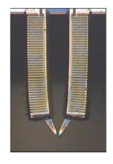
SU-8: negative photoresist, spin coated, thermally and mechically stable
