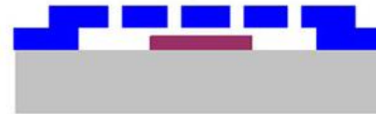
(e) Releasing the sacrificial layer.
