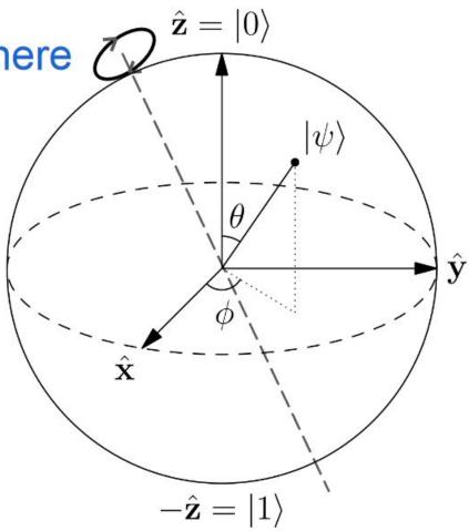
Exponentiate the Z operator to rotate by an arbitrary angle around the Z axis.
