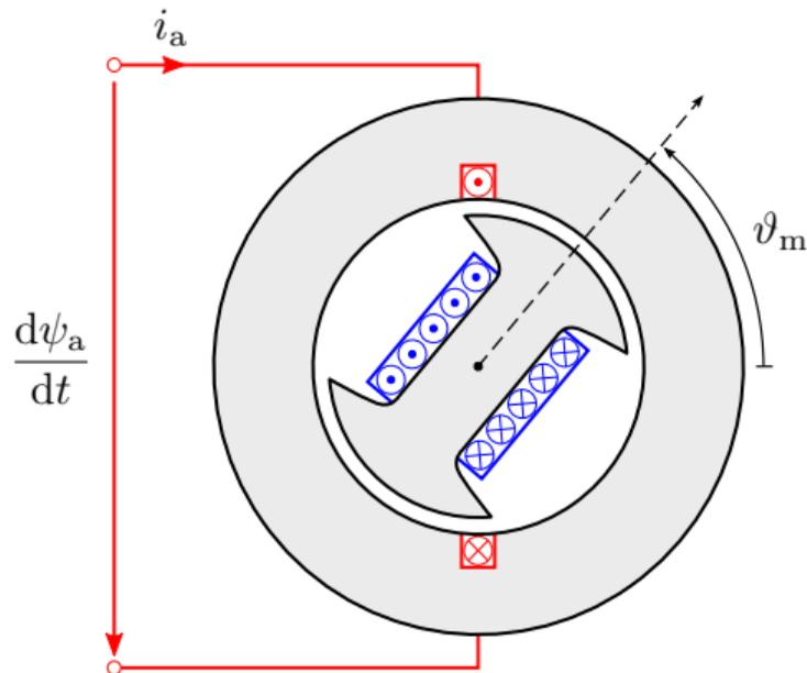
The self-inductance  $L_a$  of the ideal full-pitch coil is constant, independent of the rotor position  $\vartheta_m$ . If the effect of the stator slots on the airgap function were taken into account,  $L_a$  would depend on  $\vartheta_m$  (but not much).
