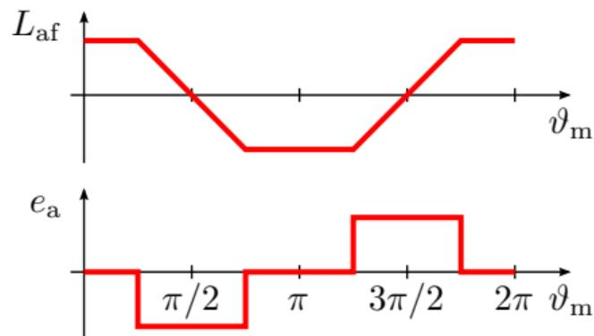
Single-Phase Machine With a Field Winding
