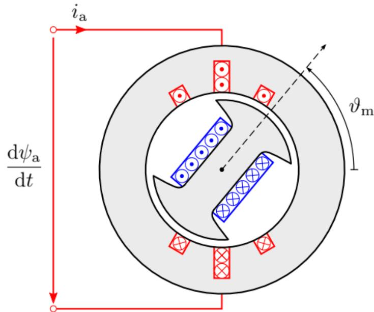
It can be noticed that the sinusoidal distribution of the winding increases the variation of the self-inductance  $L_a$ . The induced voltage  $e_a$  is not shown, but, naturally, it becomes sinusoidal as well.
