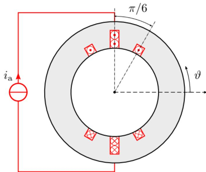
Example stator winding with  $n_a$  turns<sup>1</sup>
