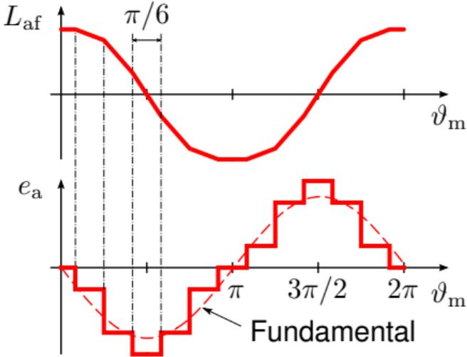
Single-Phase Machine With a Field Winding
