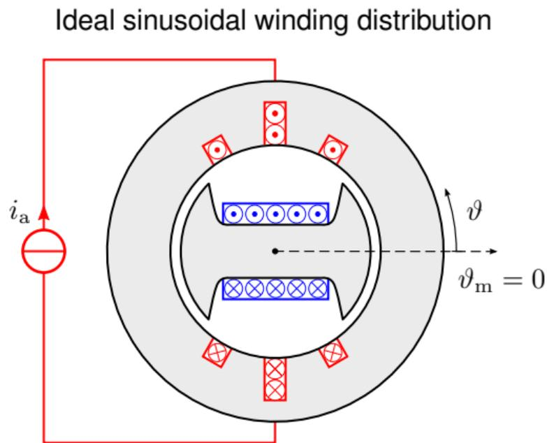
It is worth noticing that only the fundamental space component of flux density produces a net flux linkage in the sinusoidally distributed stator winding. This fact can be realized based on the flux linkage expression given earlier.
