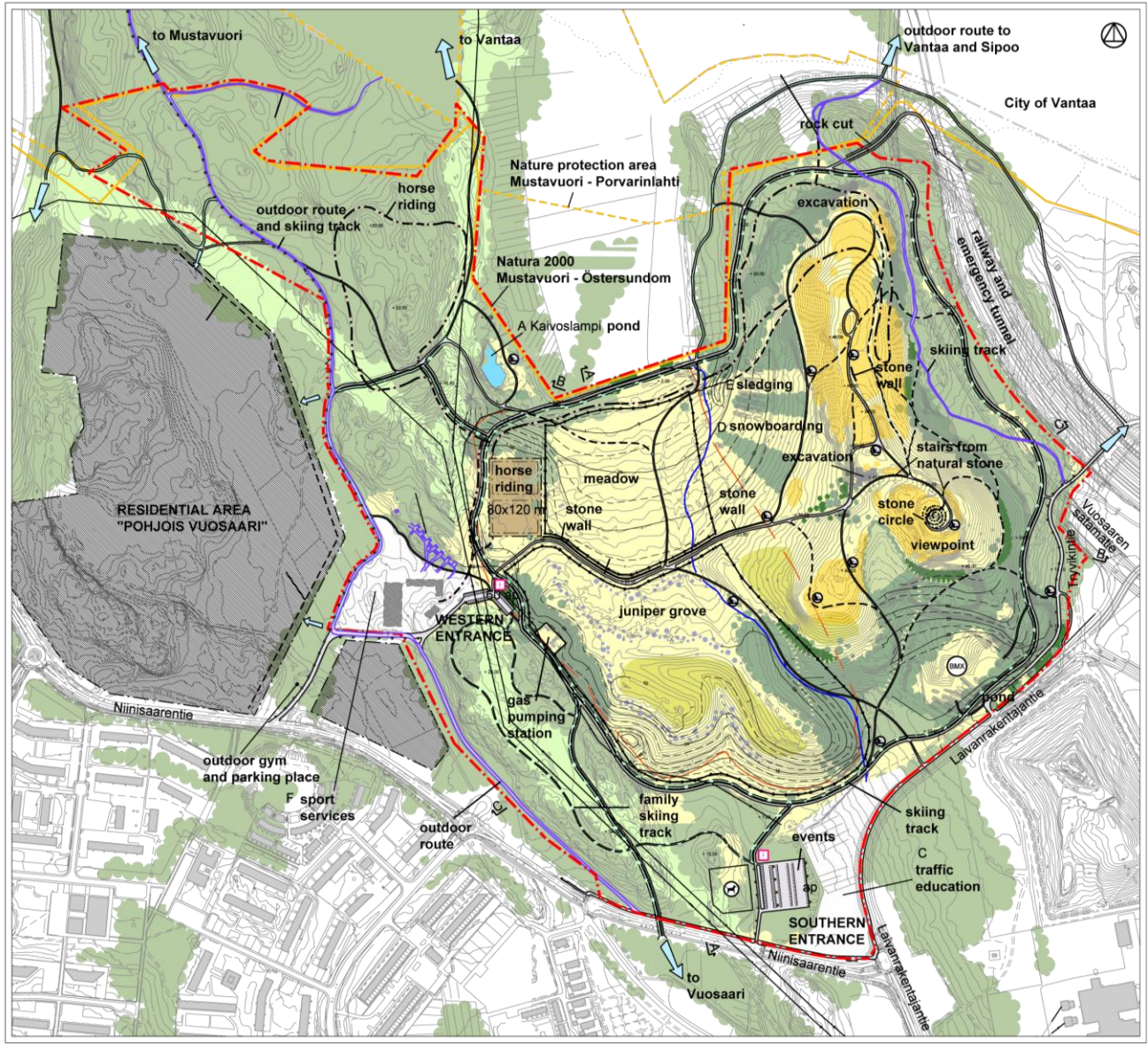
Figure 12. The General Landscaping Plan of Vuosaari landfill site integrating different activities and values (Helsinki City 2004).
