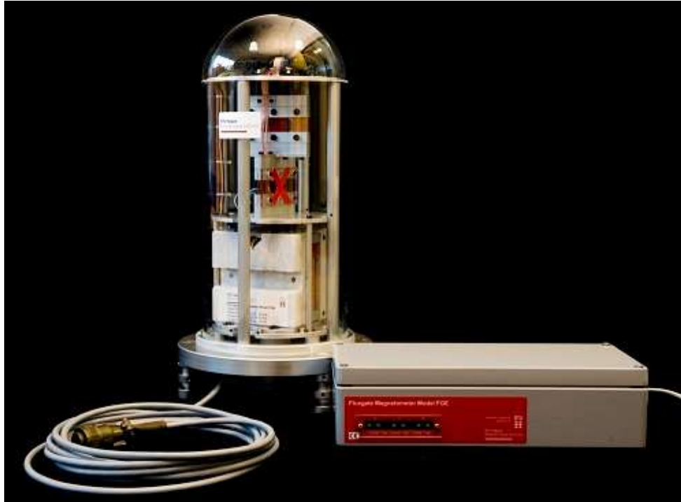
Flux gate magnetometer for scientific measurements
