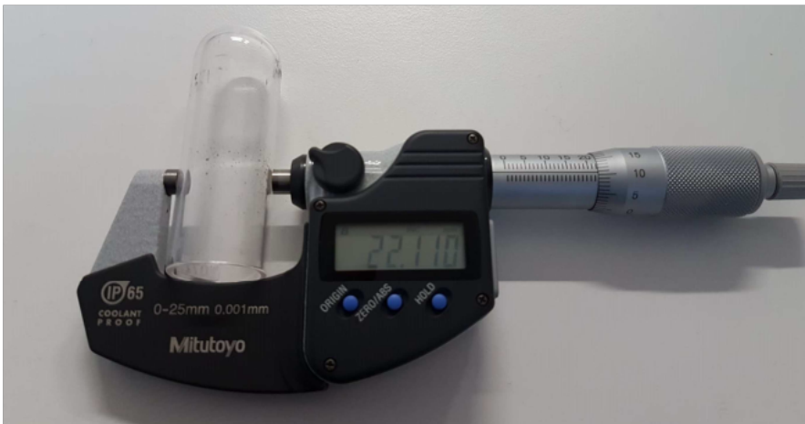
Figure 7 Cylinder outer diameter measurement
