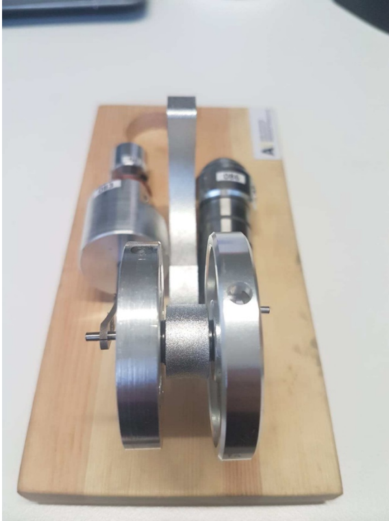
Figure 18 Flywheels, displacer piston, and power piston assembly.
