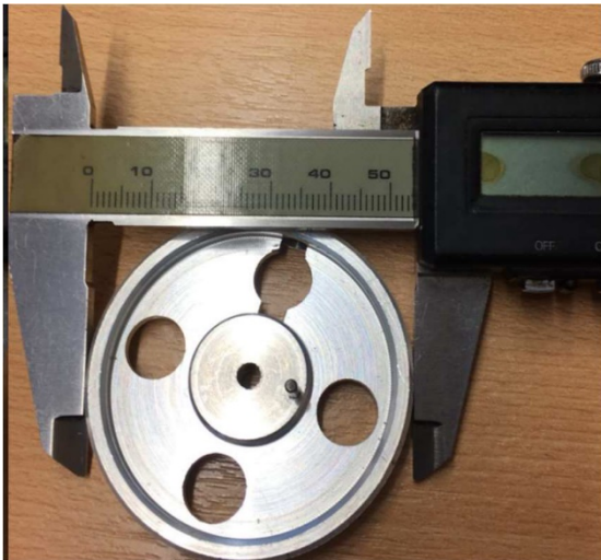
Figure 14 Flywheel diameter measurement
