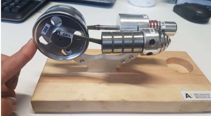
Figure 20 Flywheels, displacer piston, and power piston assembly.
