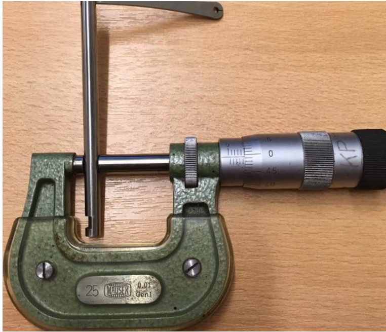
Figure 9 Micrometer measurement of displacer rod diameter
