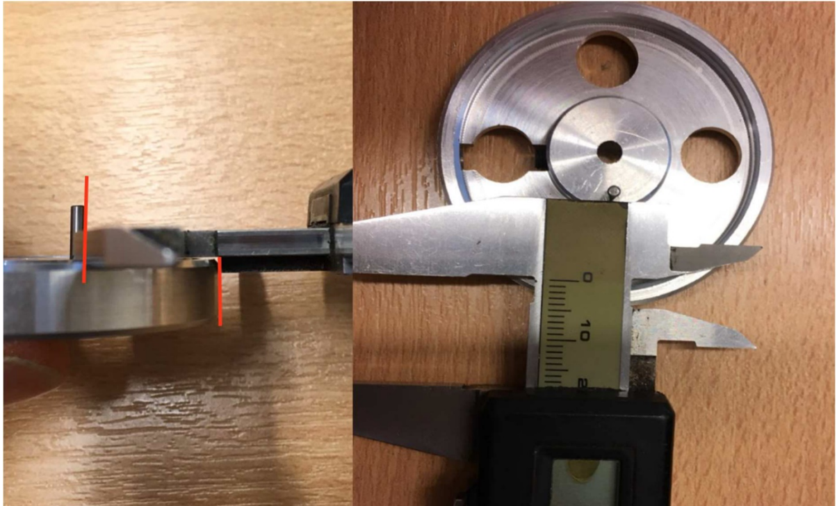
Figure 12 Pin location measurement
