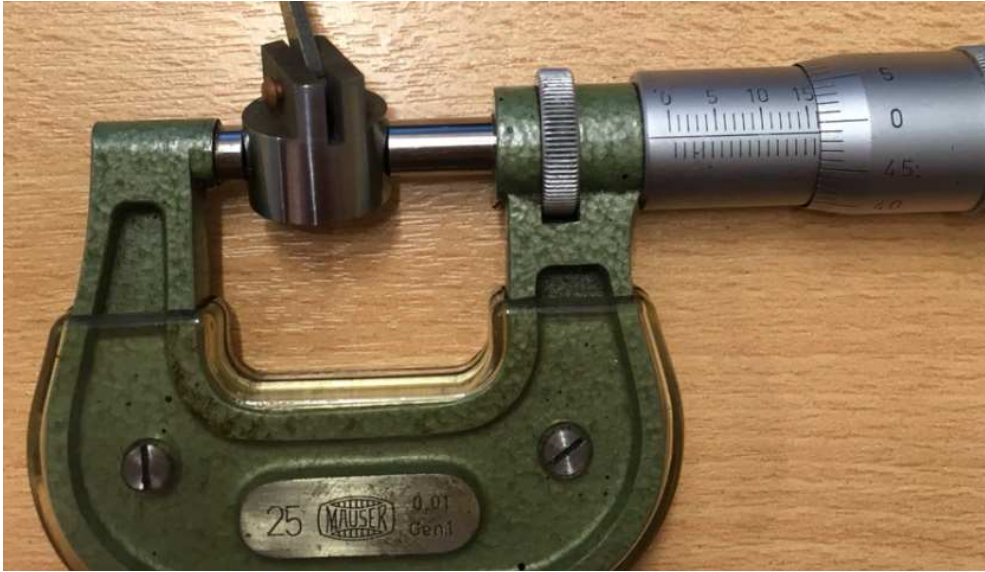
Figure 10 Power Piston diameter measurement
