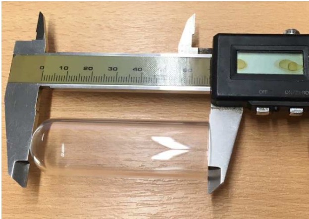
Figure 8 Cylinder length measurement
