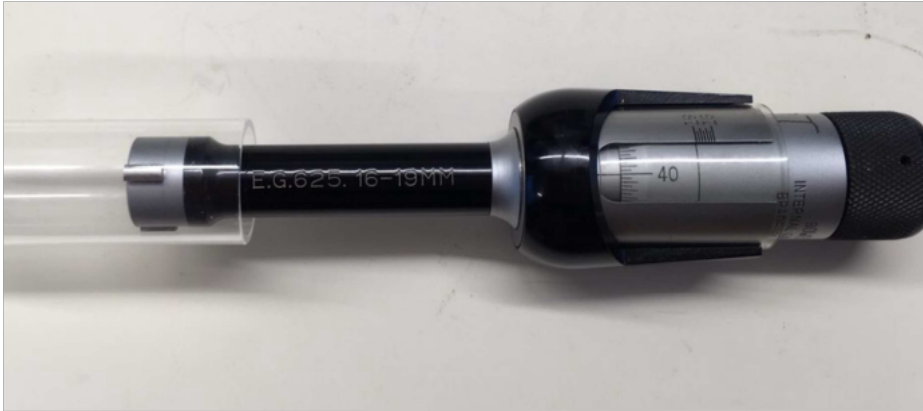
Figure 6 Cylinder diameter measurement
