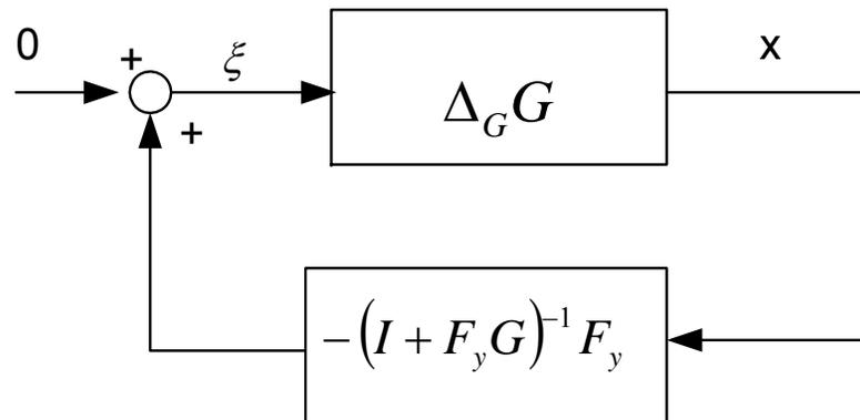
The "Small gain theorem" guarantees that the closed loop is stable, if subsystems are stable and the gain of their product
