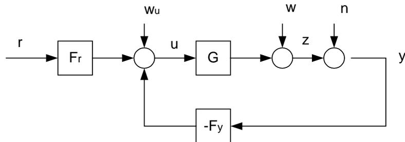
Suppose that the control, load and measurement disturbances are all zeros. Let there be modeling error in the process transfer function  $G$  such that the real process is defined as
