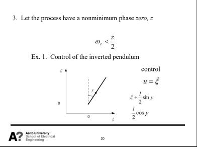
Dynamic equations  $F \cos y - mg = m \frac{d^2}{dt^2} (\frac{l}{2} \cos y) = m \frac{l}{2} (-\ddot{y} \sin y - \dot{y}^2 \cos y)$   $F \sin y = m\ddot{\xi} + m \frac{d^2}{dt^2} (\frac{l}{2} \sin y) = mu + m \frac{l}{2} (\ddot{y} \cos y - \dot{y}^2 \sin y)$ By eliminating  $F = \frac{l}{2} \ddot{y} - g \sin y = -u \cos y$ and linearizing with respect to small deviations  $G(s) = \frac{-2/l}{s^2 - \frac{2g}{l}}$
