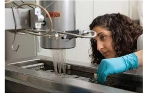
loncell production at Aalto CHEM: cellulose solution is pressed through the nozzles into a spinning bath, and fibers are formed
