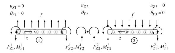
Element contributions of the two xz – plane bending beams (formulae collection) and the equilibrium equations of node 2 are (notice that the distributed force in the element contribution is the transverse component in the material system associated with beam)
