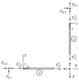
Element contributions are written in terms of the force and displacement components in the structural system. All the components of the elementwise material coordinate systems need to be expressed in terms of those of the structural system before writing the equilibrium equations. In this case, the relationships between the material and structural system can easily be seen from the free body diagram ( $F_{x1}^1 = F_{X1}^1$ ,  $F_{x1}^2 = -F_{Y1}^2$ , etc.)
