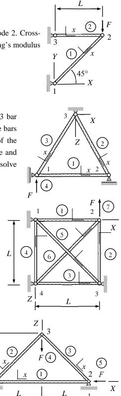
5. Determine the nodal displacements, when force *F* is acting on the structure as shown in the figure. The cross-sectional area of all the bars is *A* and the Young's modulus of the material is *E*. Use the principle of virtual work.
