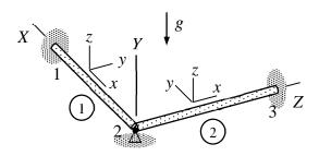
Determine the horizontal and vertical displacements of node 2. Crosssectional area of bar 1 is  $\sqrt{2}A$  and that of bar 2 is A. Young's modulus of the material is E.
