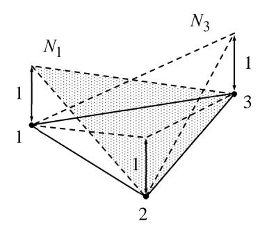
Triangle element is the simplest element in two dimensions. Division of any 2D domain into triangles is always possible, which makes the element quite useful.
