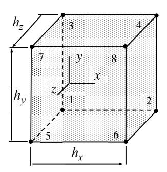
Bi-linear and tri-linear shape functions of 2D and 3D cases are products of the linear shape functions of the 1D case.
