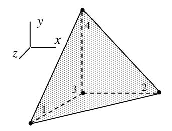
Tetrahedron is the simplest element in three dimensions. Division of any 3D domain into tetrahedrons is always possible, which makes also this element quite useful in practice.
