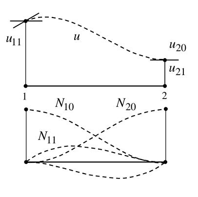
In xz-plane bending  $u = u_z$  and  $du / dx = -\theta_y$ , in xy-plane  $u = u_y$  and  $du / dx = \theta_z$ . Week 46-40 • In one-dimensional case, the brute force approach works. Let us collect the coefficients of the monomials of the shape functions into a matrix, and use the definition of the shape functions
