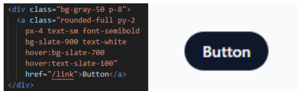
Figure 3. Example of Tailwind CSS. Left is CSS and right is the render. Each class applies a small set of CSS rules. For example the class ".py-2" is equal to the following: "padding-top: 0.5rem; padding-bottom: 0.5rem;"
