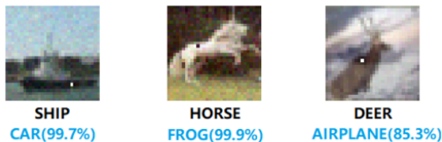
Figure 3: An optimally placed one-pixel perturbation causes a DNN to confidently misclassify an image of a ship as a car, etc. Adapted from [8].
