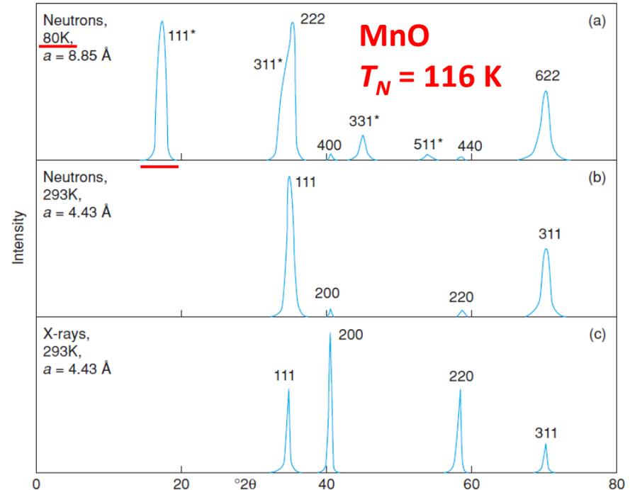
**Figure 5.26** Schematic neutron and powder XRD patterns for  $\text{MnO}$  for  $\lambda = 1.542 \text{ \AA}$ . Peaks are assigned Miller indices for the cubic unit cells given. Neutron data adapted from Shull, Strauser and Wollan, *Phys. Rev.*, 83, 333, © 1951 American Physical Society.
