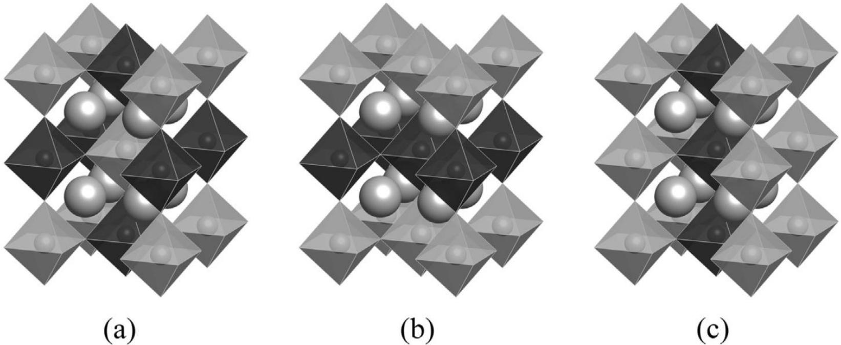
**Fig. 1.** Different  $B$ -site cation orderings found in  $A_2B'B''O_6$  perovskites: (a) rock-salt, (b) layered and (c) columnar order.
