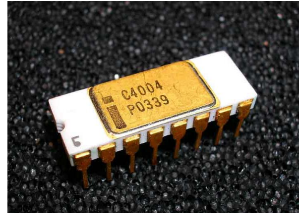
Intel 4004, the first commercial microprocessor (1971)
