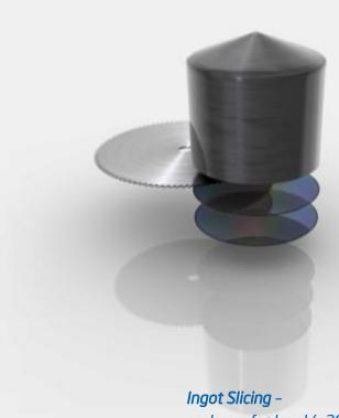
scale: wafer level (~300mm / 12 inch)
