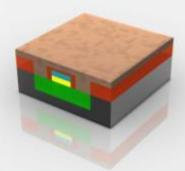
After Electroplating – scale: transistor level (~50-200nm)
