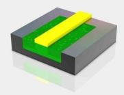
Washing off of Photo Resist – scale: transistor level (~50-200nm)
