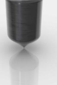
Mono-crystal Silicon Ingot – scale: wafer level (~300mm / 12 inch)
