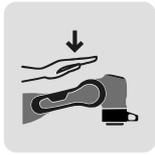
'User Interaction' enables Panda to wait for a haptic confirmation by the user. After successfully triggering a haptic gesture in one of the configured directions, the App is closed and the following App will be executed.
