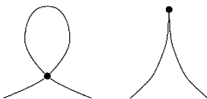
Figure 13.5. Typical singular points: (left) self-intersection, (right) cusp.
