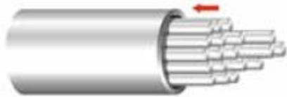
2. Multifilamentary architecture provides flexibility
