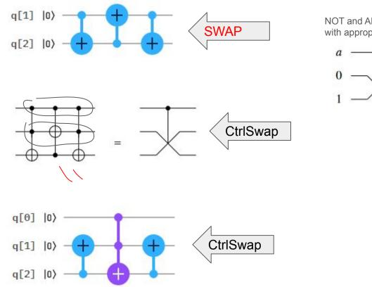
NOT and AND gates can be built from Fredkin gates with appropriate patterns of inputs
