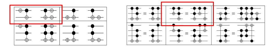
Equivalences between reversible circuits -> Can be used for circuit optimisation
