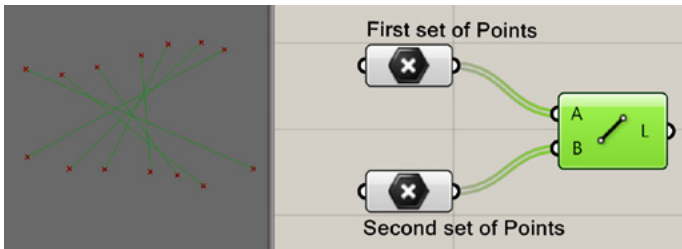
Fig.3.15. There are two lists of points and we want to connect them together by lines but when I connect them we see that the order of points in lists are not the same and what we get is not what we want. Even in this very simple example we see that some sort of data management is needed in order to get the appropriate result.
