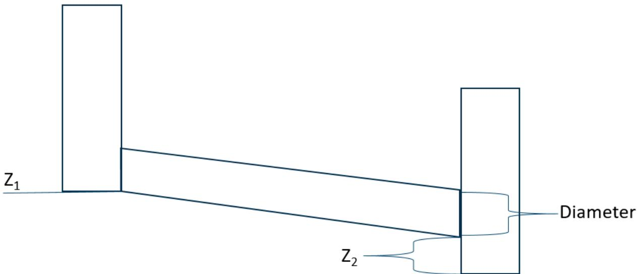
Figure 2: Pipe physical attributes (Z2 - pipe offset).
