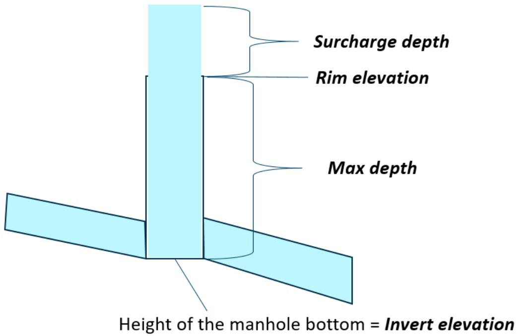
Figure 1: Junction (Manhole) physical attributes.
