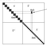
A non-zero sub-matrix, if a point *j* is visible in an image *i*
