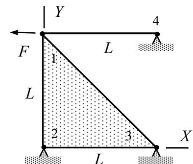
the bar  $A$  are constants. Determine displacement components  $u_{X1}$  and  $u_{Y1}$  of node 1 by using a linear bar element and a linear plane-stress element.
