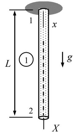
Consider a bar of length  $L$  loaded by its own weight (figure). Determine the displacement  $u_{X2}$  at the free end. Start with the virtual work density expression  $\delta w_{\Omega} = -(d\delta u / dx)EA(du / dx) + \delta u f_x$  and approximation  $u = (1 - x / L)u_{x1} + (x / L)u_{x2}$ . Cross-sectional area  $A$ , acceleration by gravity  $g$ , and material properties  $E$  and  $\rho$  are constants.
