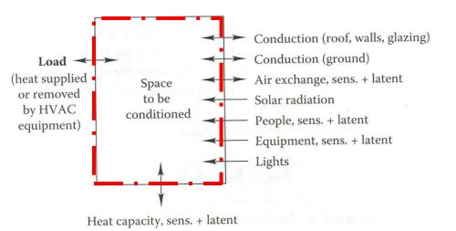
NOTE: Heating and cooling loads (gains) are expressed either as power [(k)W] or energy [(k)Wh] and the included energy needs are different. 1 kWh = 3.6 MJ
