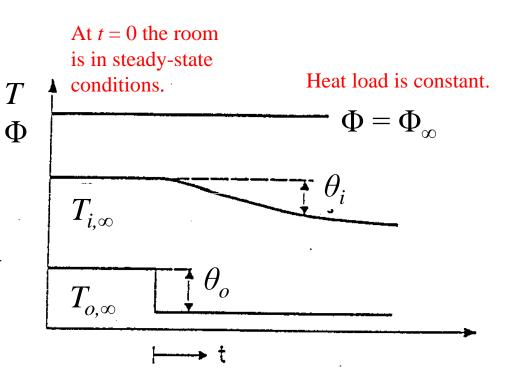
$$T_{i,n} = T_{i,n-1} + \frac{G_{tot}}{C_{tot}} \left(T_o - T_{i,n-1}\right) \Delta t$$
