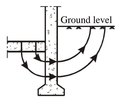
**Rule of thumb: Heat transmission to ground is constant 5 W/m<sup>2</sup> throughout a year with a good accuracy.**
