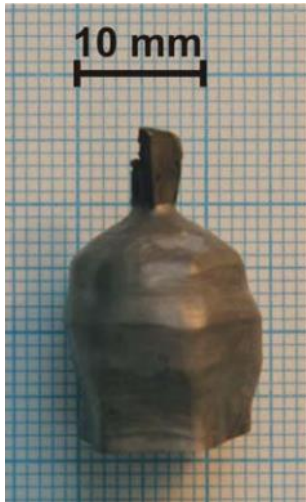
13 gram single crystal of \text{Ba}_8[\text{Ga}_{16}\text{Ge}_{30}]
