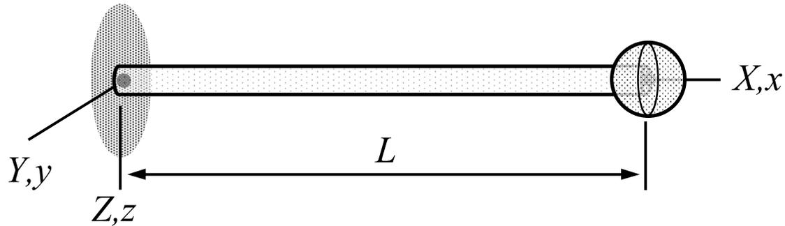
**Answer**  $\omega_3 = \omega_4 = \sqrt{2 \frac{EI}{mL^3}}$ ,  $\omega_5 = \omega_6 = \sqrt{30 \frac{EI}{mL^3}}$ ,  $\omega_2 = \sqrt{10 \frac{GI}{mL^3}}$ , and  $\omega_1 = \sqrt{\frac{EA}{mL}}$
