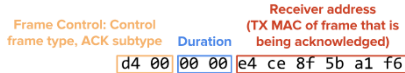
Figure 15. Acknowledgment of the 802.11 frame
