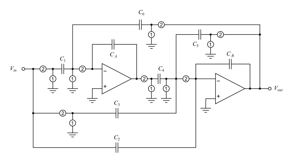
Problem is the loop connection of the two integrators during phase (2)
